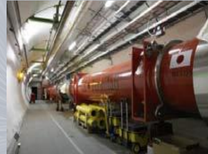
LHC superconducting magnets (超伝導磁石) by TOSHIBA, Furukawa(古河電気) and many [photos from ATLAS-Japan group]
